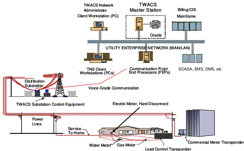
Outbound signalling is communication from the substation to the end-point devices and inbound signalling for end-point device communication detected at the substation. This is a low bandwidth technology that reliance on clever use of concurrency techniques to deliver its service. This is a proprietary technology.
