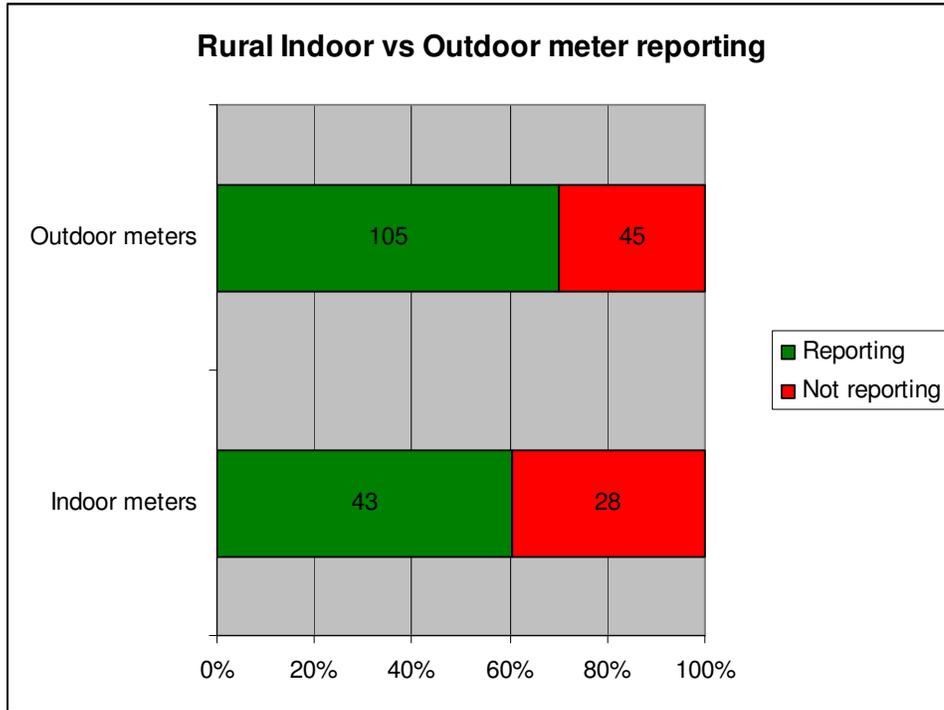
Note that in the case of outdoor meters, the orientation of the meter cabinet relative to other meters determines whether the meter will mesh. Unfortunately this is entirely random and impossible to predict or model without surveying each and every meter location
